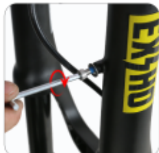
Loosen the screws on both sides of the front fork
