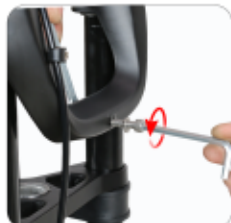
Loosen the front fork screws with a hexagonal screwdriver
