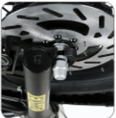
Align the protruding part of the nut washer with the bayonet, and tighten the screw
