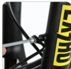
Tighten the screws on left sides of the front fork
