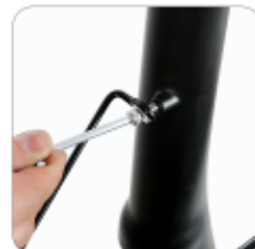
Tighten the screws on right sides of the front fork
