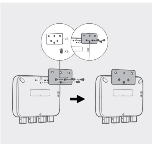
2. Install two M6\*20 in two holes of the installation board, and tighten M6 nuts on them.
