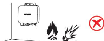
The IP rating of the microinverter is IP 67, hence, it can be installed either indoors or outdoors. However, the EcoFlow portable power station is not waterproof. If your system includes a portable power station, keep both of them indoors.
