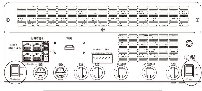
1. Power Switch: Control power supply for the unit
