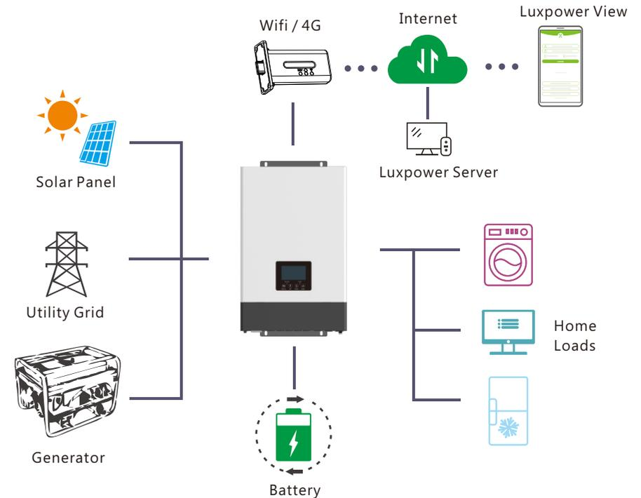
SONAR series is a multifunctional, high frequency pure sine wave off grid solar inverter, features:
