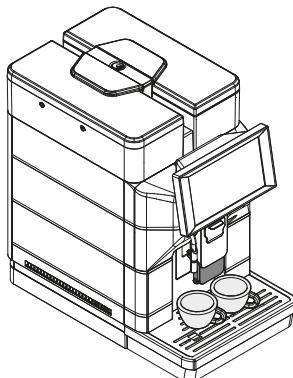
Push the dispensing spout towards the machine interior to its limit stop, to allow the use of tall glasses or MUGS. In this case, you can just brew one product at a time.
