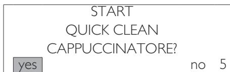
Proceed as follows to perform the rinse cycle: Select "YES" and press the "OK" button. The following screen is displayed:
