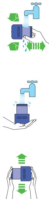
Wash the outside of the filter, rubbing with your fingers to remove the dirt.
