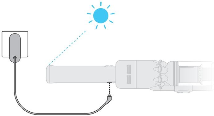
The LED light on the end of the handle will flash when the power is running low and to charge your battery.
