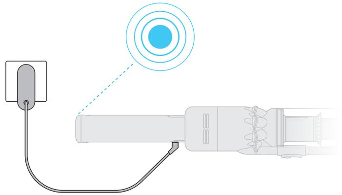
It can take up to 3.5 hours to fully charge your battery. Your battery has been designed to be left on charge.
