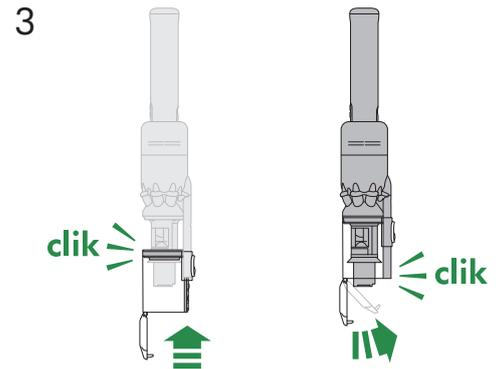
To close the bin, push the bin base upwards until the bin and lid both click into place. Reconnect the wand.
