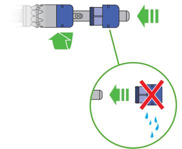
To refit your filter, slide it onto the handle, slide it onto the handle and turn it clockwise until it clicks into place.
