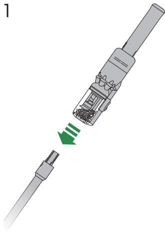
Press the red wand release button and pull the wand away from the bin.
