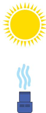
Shake to remove any excess water and place it with the filter end up. Leave for at least 24 hrs to dry.
