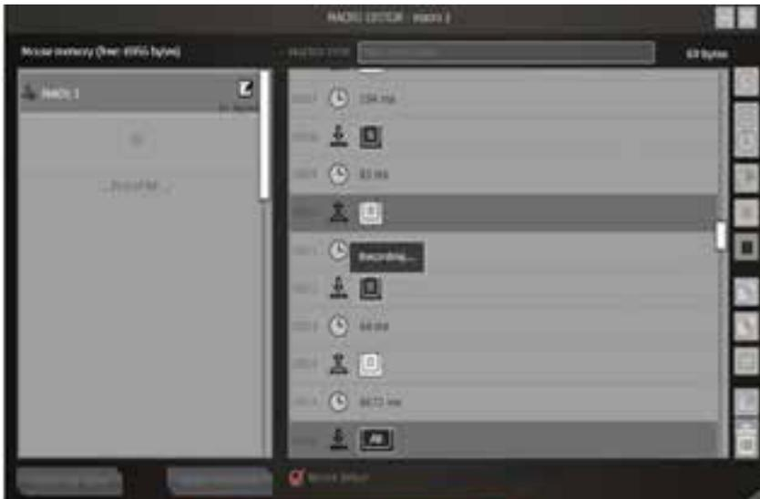
You may edit the macro using the *delay*, *keyboard*, *mouse* or *scroll command*, or *mouse movement*.
