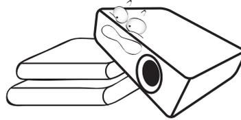
13. Do not stand the projector on end vertically. Doing so may cause the projector to fall over, causing injury or resulting in damage to the projector.
