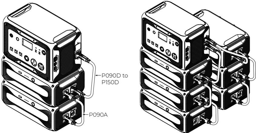
**Note:** The AC500 can work with B300K, B300S and B300 expansion batteries simultaneously. To connect them:
