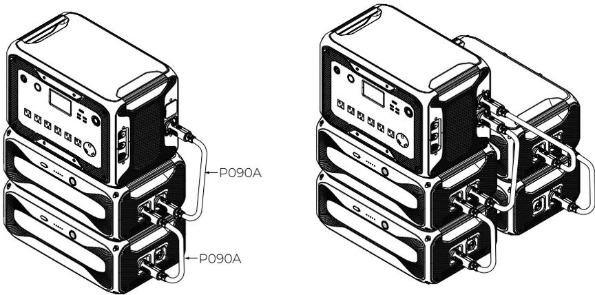
**Note:** The AC300 can work with B300K and B300 expansion batteries simultaneously using P090A battery expansion cables.
