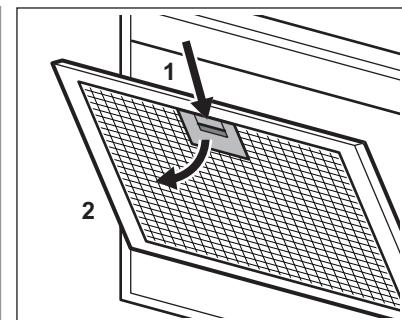
2. Slightly tilt the front of the filter downwards (2), then pull.
